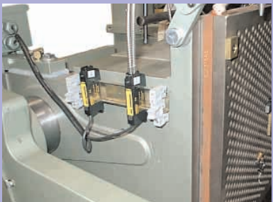
Fiber optic signal pick up device mounted to the side of the press (shown on EHF).
